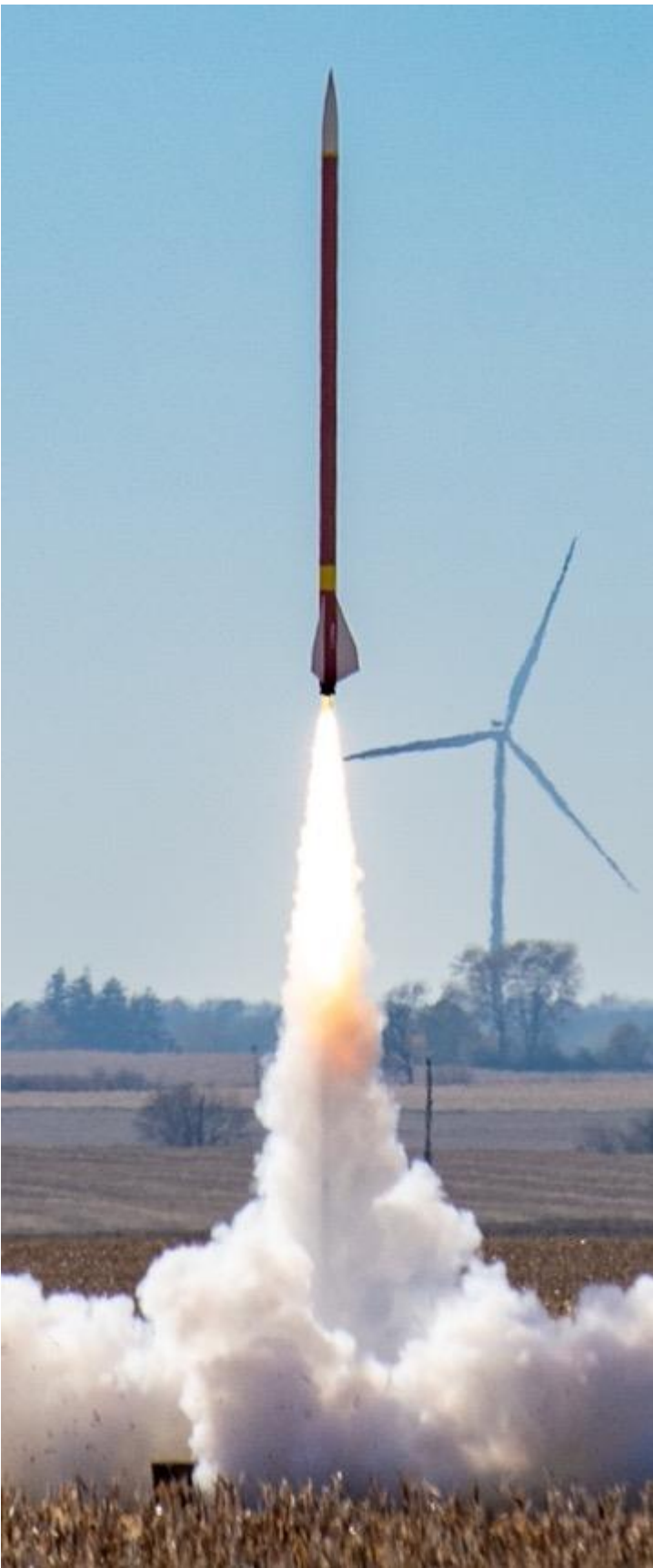
Also on Saturday, Chris Pearson flew his upscaled 5.5" North Coast Rocketry "Lance Beta" with a 54mm Research J480 motor using NASSA K2 Fast propellant. It hit 2000 feet and landed 50 feet from where Chris was standing.
