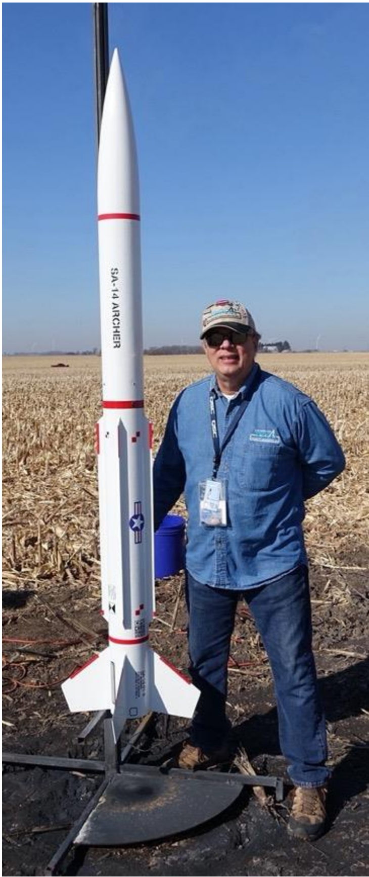
On Saturday, Chris Pearson flew his upscaled 5.5" North Coast Rocketry "Archer SA-14" with a 54mm Research J480 motor using NASSA K2 Fast propellant. It did a respectful 2200 feet and landed between the B and C cells of the launch range.
