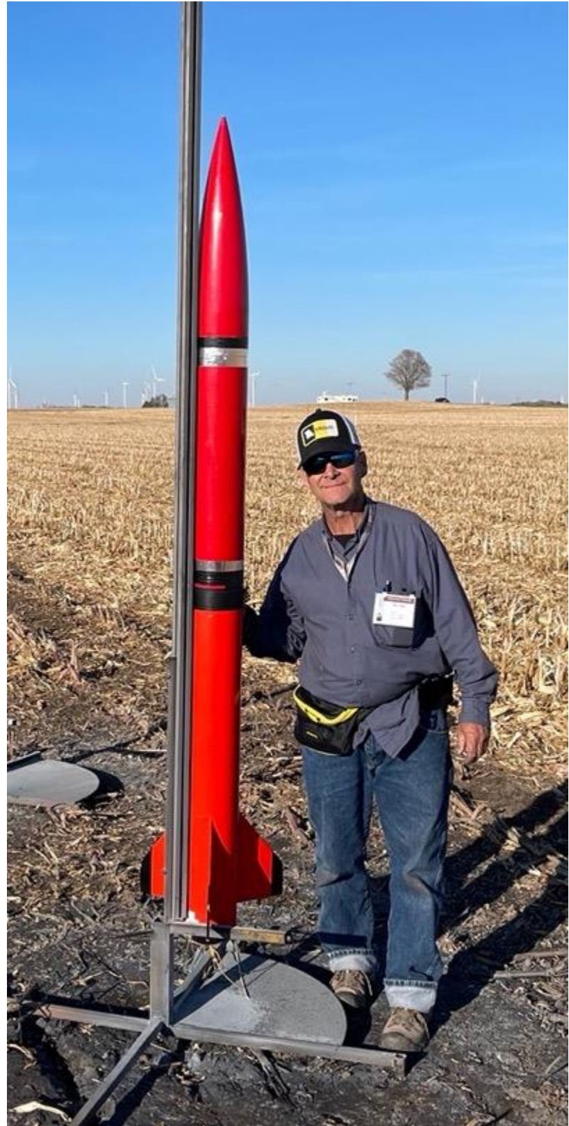
Mark also flew his scratch-built 5.5" "Cheeto" on a three-grain 75mm Research L1175 flying to an altitude of 6522 feet.
