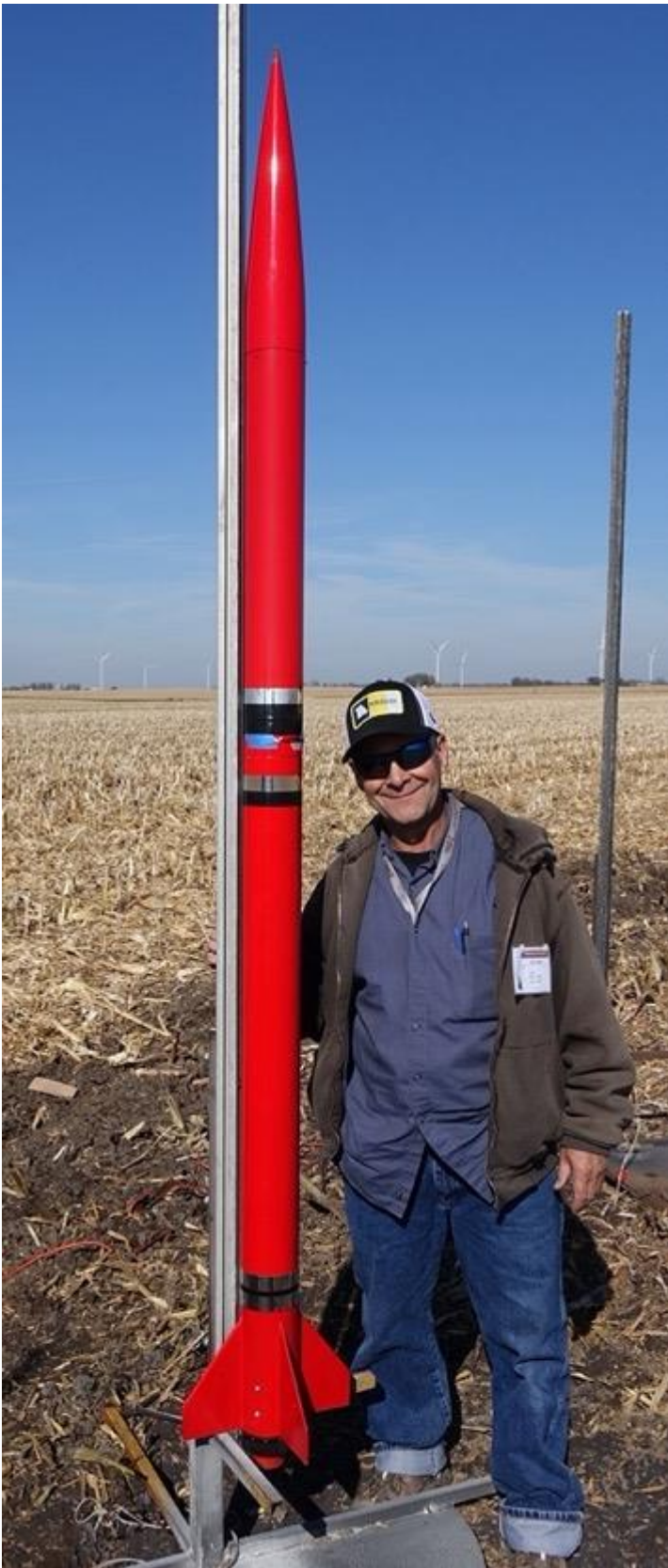
Mark Coburn flew his 4" "Arcas" with a Research 4 grain 75mm L1500 using NASSA K-2 Fast propellant to an altitude of 11,200 feet.
