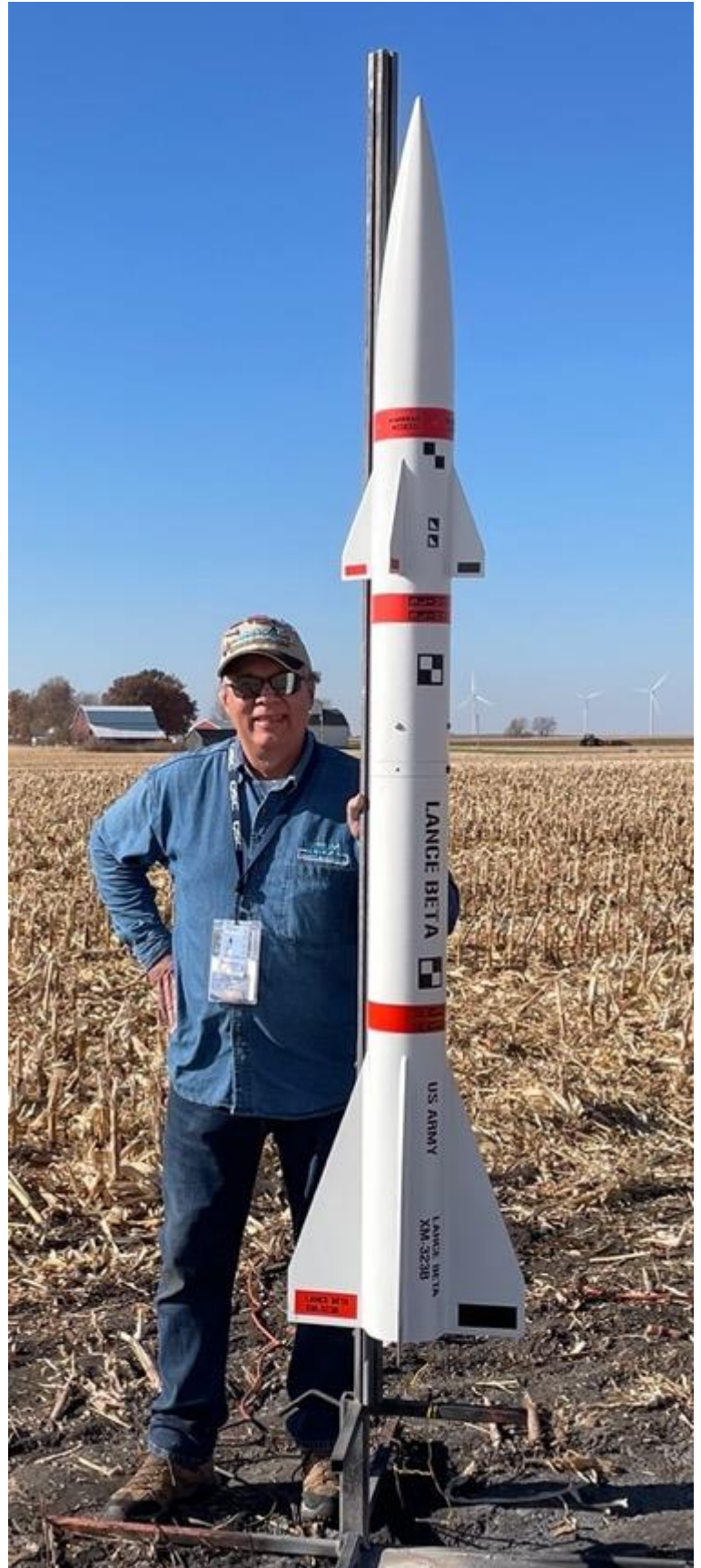
Also on Saturday, Chris Pearson flew his upscaled 5.5" North Coast Rocketry "Lance Beta" with a 54mm Research J480 motor using NASSA K2 Fast propellant. It hit 2000 feet and landed 50 feet from where Chris was standing.
