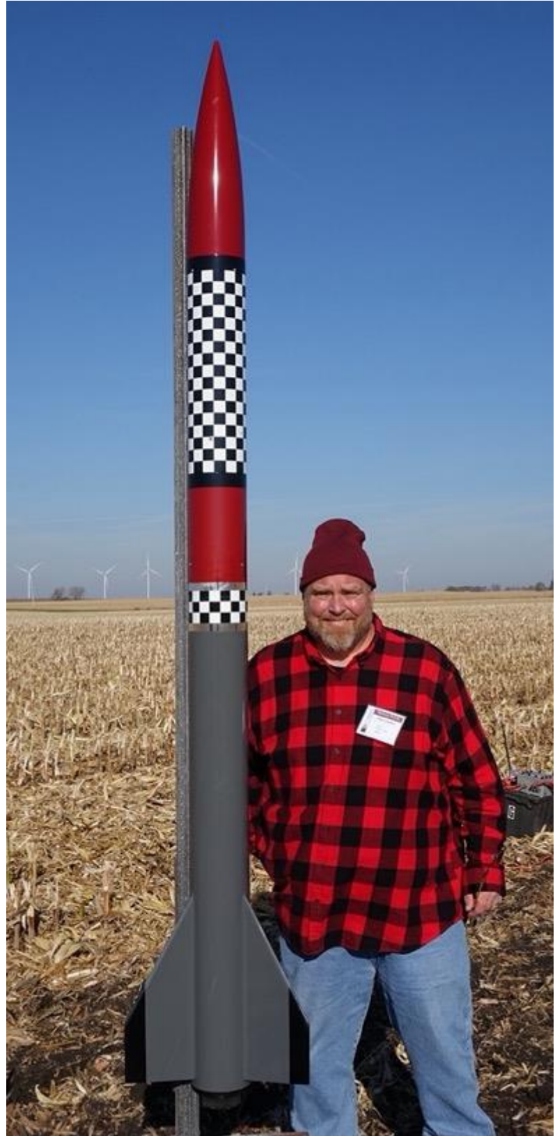
On Saturday Andrew flew his "Petunia" again this time on a 75mm 3-grain red Research motor which he guessed was about a L1400. It flew to 5875 feet and was recovered close to the pads.
