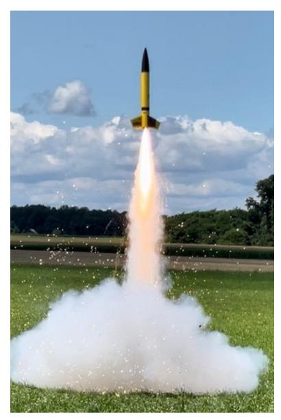
Pete Taran's 4' LOC/Precision "Goblin" (left) which he used for his Level 2 Certification flight. He flew it with an AT J340 M sparky motor to an altitude of 3500 feet for a successful L2 cert flight!
