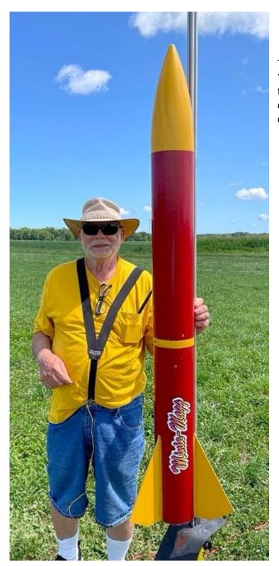
Terry Habegger (left) puts his extended LOC/Precision "Mini-Magg" which he calls his "LOC Red Rocket" on the pad. He flew it with an AT J420 R motor and was expecting an altitude of 3000 feet, but the electronics didn't deploy the recovery system.
