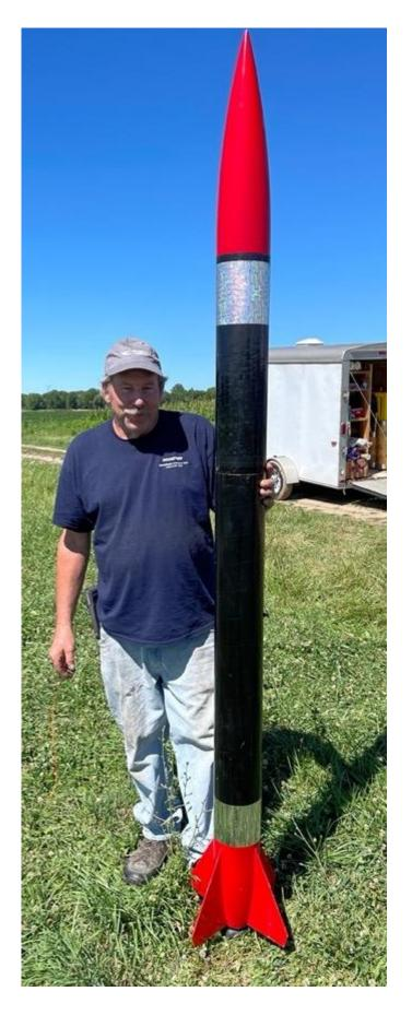
Steve Eves (above) with another of original LOC/Precision rockets from the 80's, a "Syonic" which he flew with a Research K600 motor to an altitude of 3000 feet using NASSA K2 Fast Propellant.
