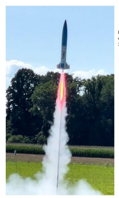
Pete Taran's 4" LOC/Precision "T-LOC" takes to the air with an AT H268 R motor which took it to an altitude of 3000 feet (left).
