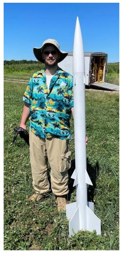
Chris Feyerchak flew his LOC/Precision "Nike-Zeus" with an electronics bay modification on an AT H180 W motor for a Level 1 certification flight to an altitude of only 632 feet! But he got the certification! Chris' flight was one of four L1 certification flights done at the launch.
